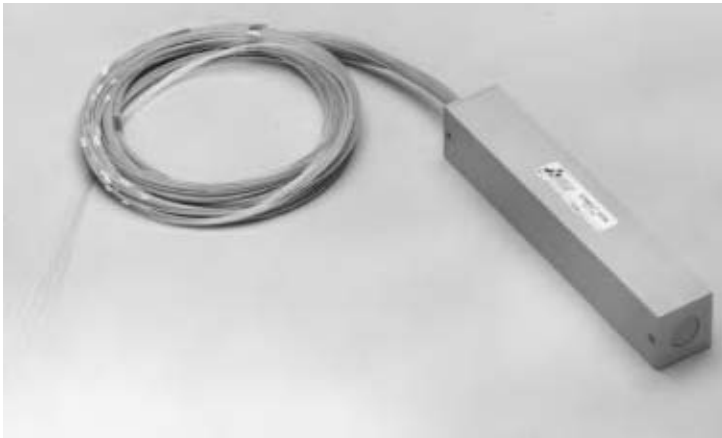
Figure 6.20 Typical diffraction grating router. 22 \times 22 Input/Output ports. Spacing between channels: 1.6, 0.8, or 0.4 nm. Physical size 234 \times 35 \times 35 . ( Source : HighWave Optical Technology. Reprinted with permission).
