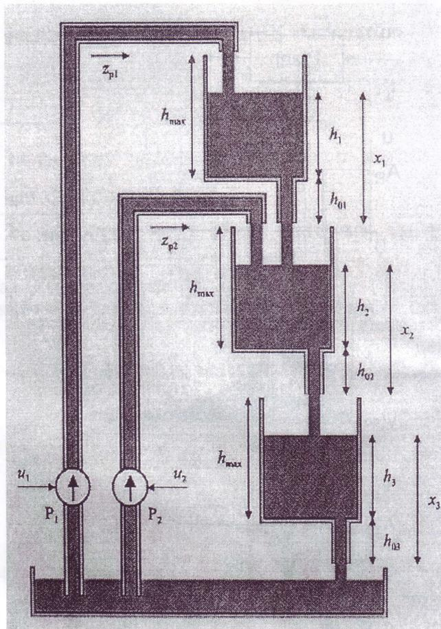
Figure 4.1. Three tank system, description of the experimental laboratory unit
