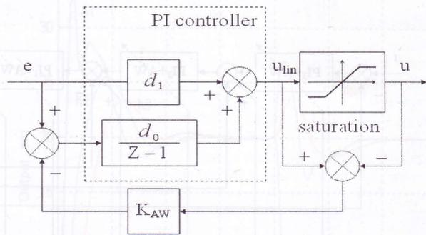
Figure 4.3. PI controller plus anti-windup structure.
