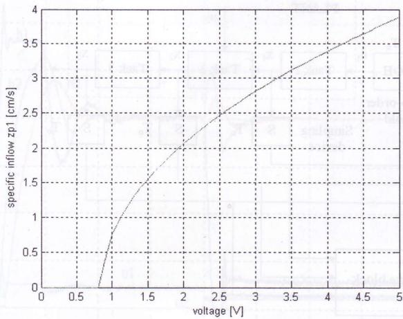
Figure 4.2. Three tank system, nonlinearity and the resulting inflow
