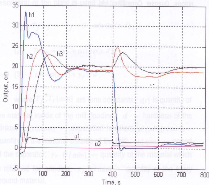
**Figure 5.4.** The real time experiment results obtained using (Hang, 1991) tuning method
