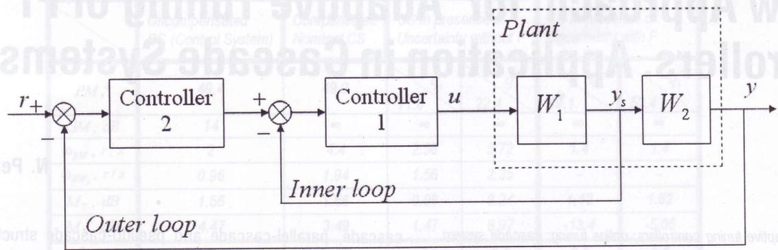
**Figure 2.1** Block diagram of a cascade control system
