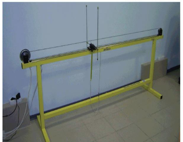
Figure 1. The inverted pendulum laboratory model
